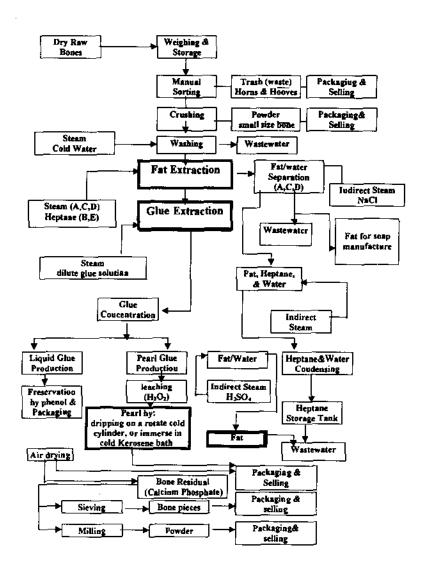
Figure 1: Schematic diagram of giue manufacturing process
